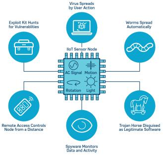
Figure 2. Various types of malware that can potentially infect an IIoT system.
