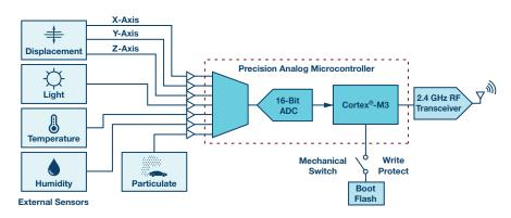
Figure 4. Physically write protecting firmware, except when performing an update, is an effective way to protect the integrity of a device.
