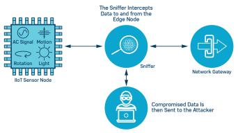
Figure 3. A Man-in-the-middle attack inserts a malicious access point between a node and a gateway.
