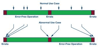
Figure 5. Exploiting small errata to force a failure 100% of the time.
